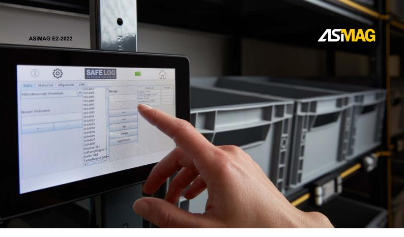
Using a unique two-conductor profile cable, ASi-5 connects the control unit with an integrated touchscreen to up to 96 receiver devices.
