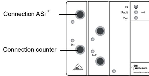
\* Remark: If you use this connection for ASi, do not connect an ASi cable to the substructure.
