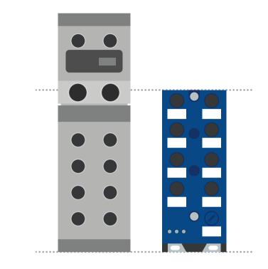
Compared with Ethernet-based fieldbus modules, similar ASi-5 modules using piercing technology are both less costly and significantly more compact.
