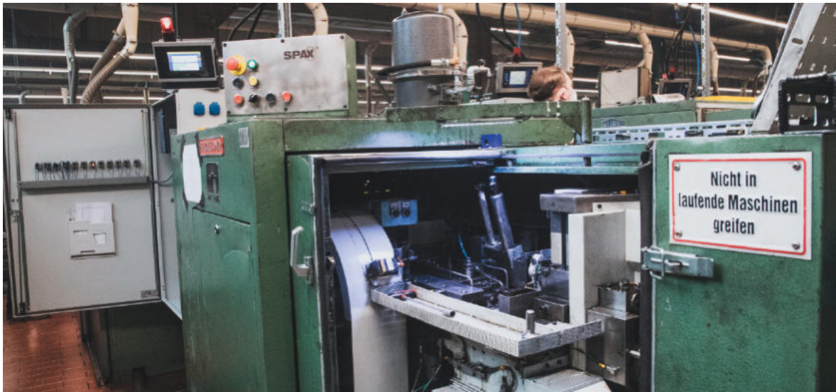
Press with control cabinet.
