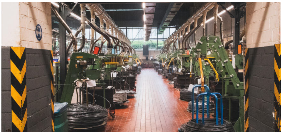
SPAX uses a variety of identical or similar machines for manufacturing screws.
