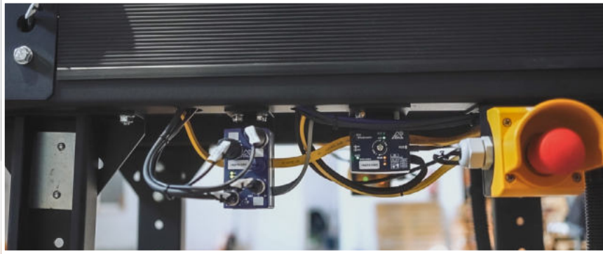
ASI-5 Motor Module BWU4246 (left) and ASI-5 Active Distributor for RGB stripes BWU4083 (right).
