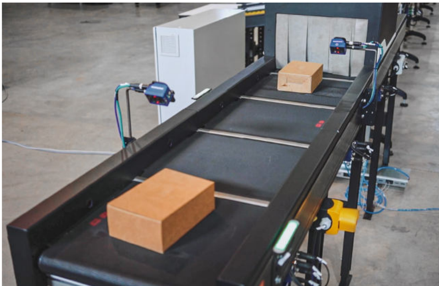
Conveyor belt with LED stripes and SKU barcode scanner (front) and CLUSTAG RFID technology.
