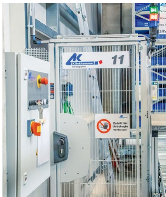
Aisle door (left), control panel with Bihl+Wiedemann safety technology
