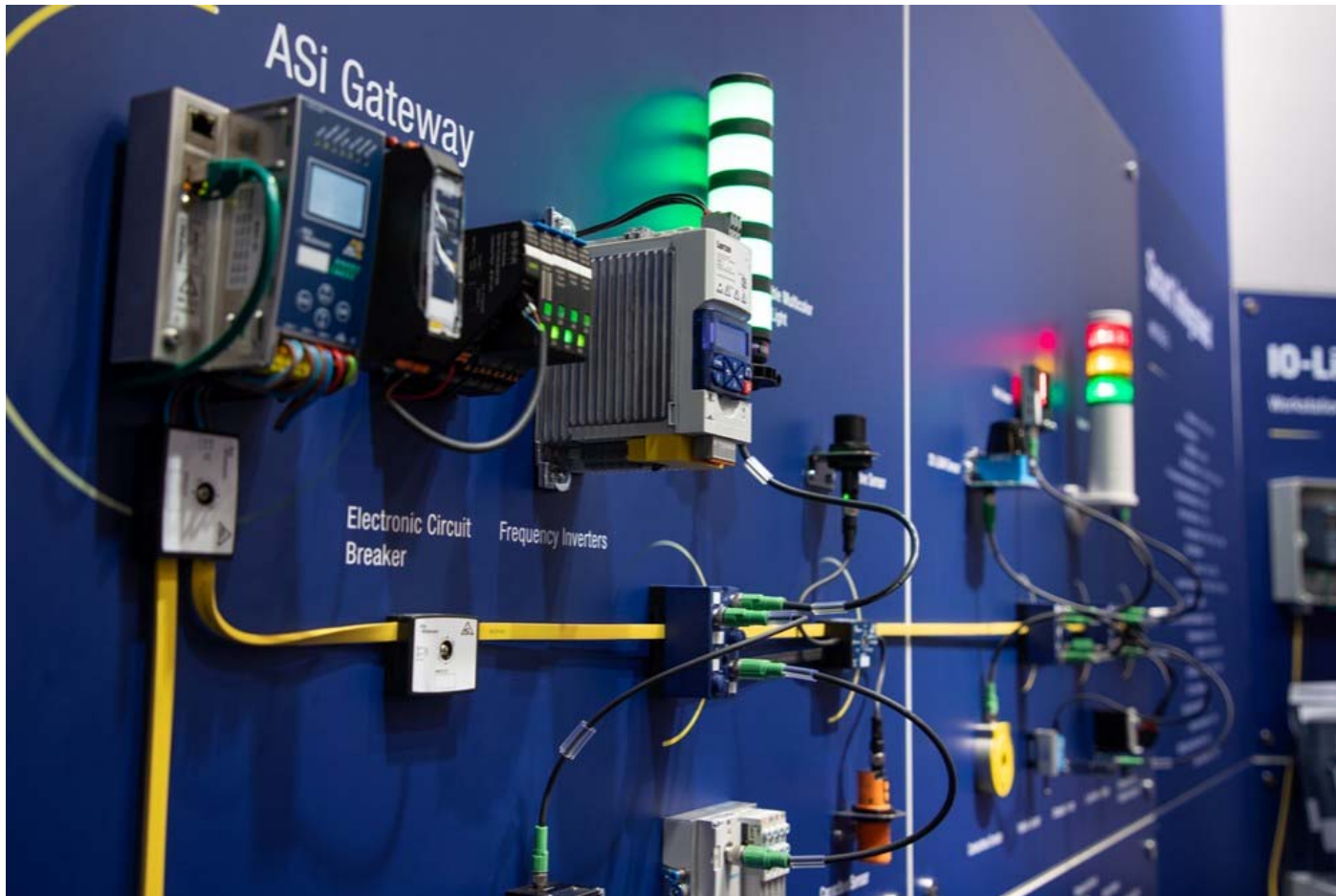
Fig.: ASi-5 makes it easy to connect a wide variety of IO-Link devices to the control system
