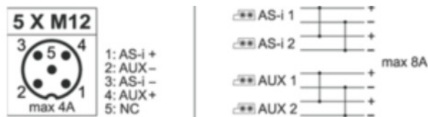
Fig. 1: Connection diagram for the M12 sockets and the flat cable branch in the new AS-i IP67 passive distributor with five M12 sockets (BW2820).
