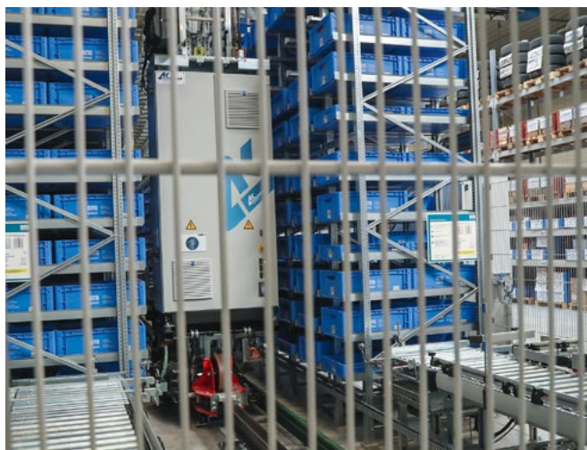
S/RM in aisle with material handling technology (left), LHD unloading a compartment (right)
