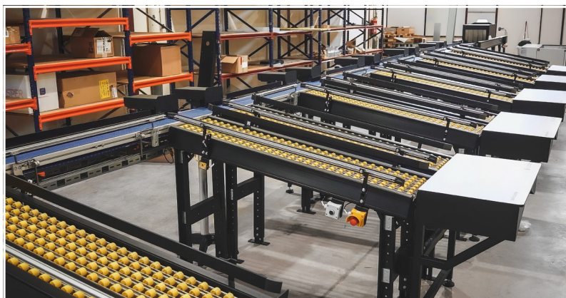
The RIELEC Fit Sorter package sorter can sort up to 1800 cartons per hour.
