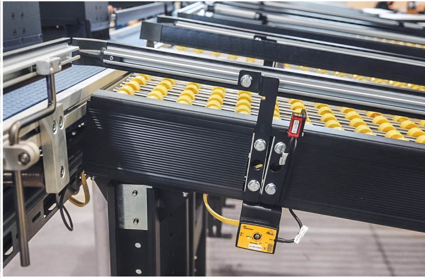
The active distributor ASI Safety (BWU3599) from Bihl+Wiedemann permits implementation of safety applications up to SIL3/PLe.
